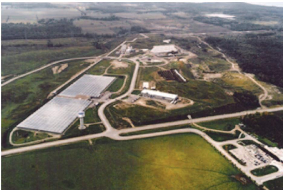
In 1996, a new oil-fired steam plant was constructed to replace the then-inoperable units of Bruce 1 to 4. This plant can deliver up to 250,000 pounds per hour of steam at a pressure of 300 pounds per square inch. This temporary arrangement is unsuitable for the longer term.
